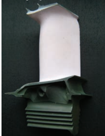
Figure 1. A low K thermal barrier coating, doped with Erbium.
