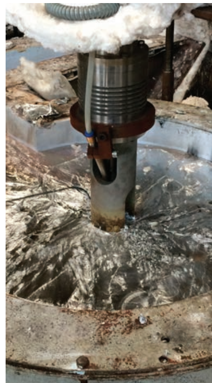
Right: Direct chill casting of a 4.5 tonne aluminium alloy billet, implementing LiME's rotor-stator high shear technology
